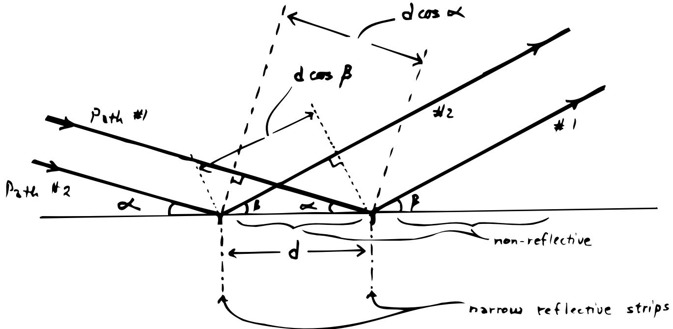
Again, the two incoming "paths" are parts of a plane wave (in phase, in your experiment, because they issue from a laser); the outgoing paths shown will be in phase as well—again forming a plane wave—if the difference between the
