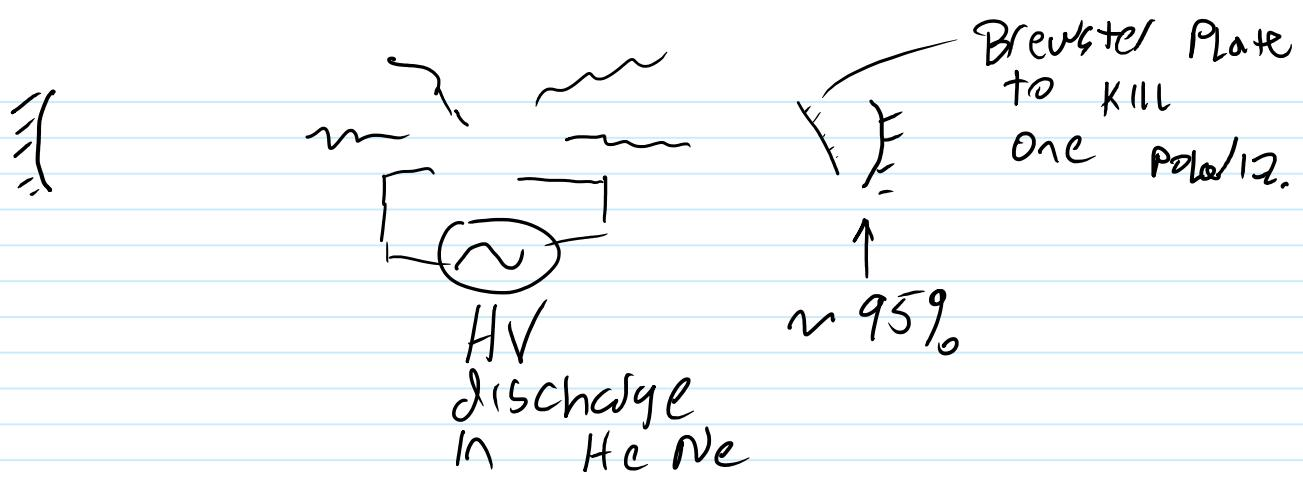
The laser cavity tube length is about 0.486 meters for the 1135p laser (you look it up). The wavelength of the laser is set by an energy transition in the HeNe gas--- 632.8 nm.
