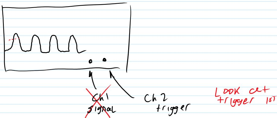
When the trigger signal reaches a level we set (voltage) then this tells the oscilloscope "start" acquiring data. We set it to acquire for 20.0ns---keep and hold, wait till ready (could be microseconds later) ---then take next pulse that triggers. If the signal is identical, it will overlay. If not---we see jitter and noise on entire pattern. So we average 512 pulses, and it really cleans up. WE THEN NEVER MOVE TRIGGER PHOTODIODE---.
