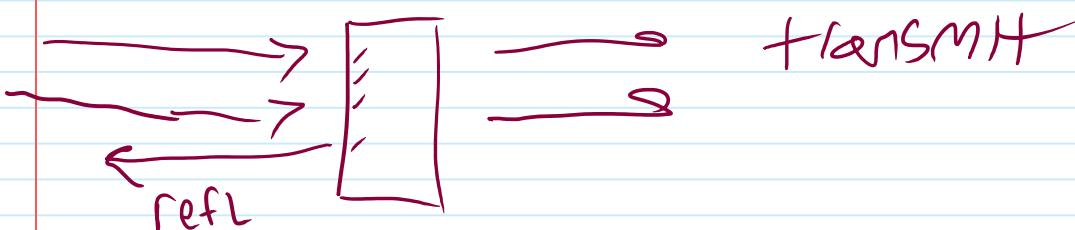
Part of the wave energy (Amplitude) passes through, and part is reflected. The waves can be brought together later at some point by using geometry and mirrors. There are many types of such "Division of Amplitude" devices. In both cases the light needs to be coherent. But here if the path difference introduced is too long---the waves will no longer be synchronized.
