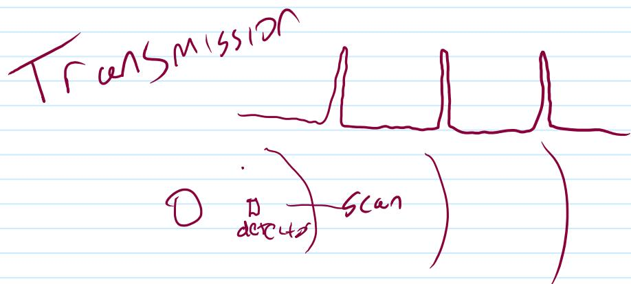
The width of a ring compared to the space between rings (free spectral range)---gives spectroscopic information of bandwidth of light spectra. Higher R leads to better resolution (narrower rings).
