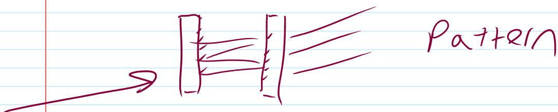
Adding a little curvature and a gain medium in the middle, turns this into a LASER.
