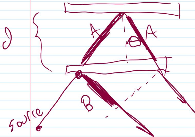
The path difference can be worked out as "2d cos(θ)". It is of note that the maximum P.D. is at the center of pattern where the angle is zero. The Zero order fringe is at 90.
